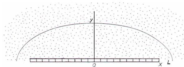
Figure 1. Condensate film flow on a finite-size horizontal plate with porous medium.
