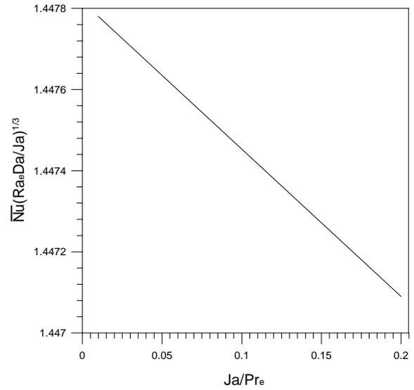
Figure 3. Dimensionless heat transfer coefficient with porous medium.
