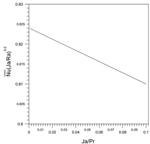
Figure 2. Dimensionless heat transfer coefficient without porous medium.
