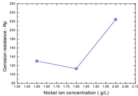
Fig. 4. The relationship between the corrosion resistance and the nickel ion concentration in the electrolyte.
