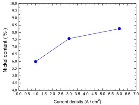
Fig. 2. The effect of the applied current density on the nickel content in the obtained Ni-Zn coating.
