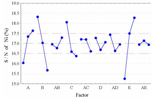
Fig. 1a. S/N ratio vs. factor effects of the nickel content in the coating.
