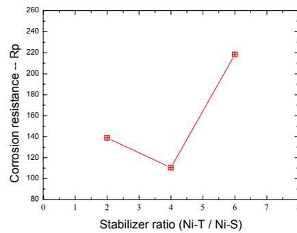
Fig. 5. The dependence of the corrosion resistance on the amount of stabilizer ratio in the electrolyte.
