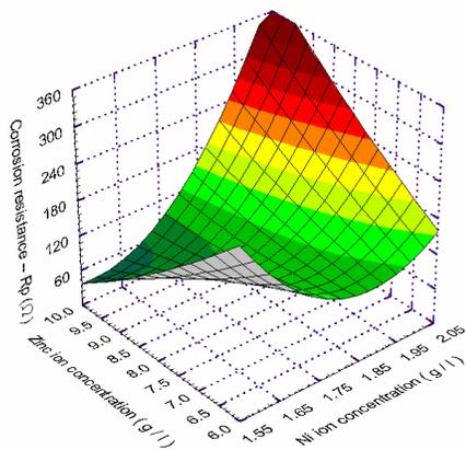
Fig. 6. The response surface shows the variation of corrosion resistance of the Zn-Ni alloy with the interaction between the concentration of nickel ion and zinc ion in electrolyte.
