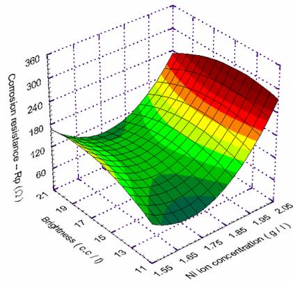
Fig. 7. The response surface shows the variation of corrosion resistance of the Zn-Ni alloy with the interaction between the nickel ion and brightener concentration.
