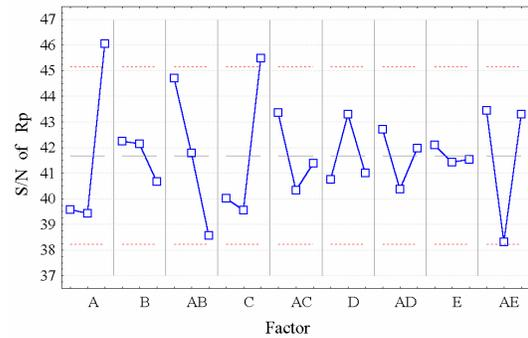
Fig. 1b. S/N ratio vs. factor effects of the corrosion resistance (Rp) of the coatings.
