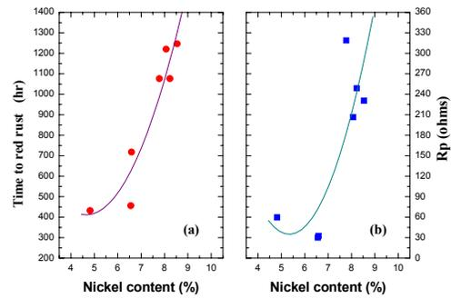
Fig 8. The relation of nickel content vs. corrosion resistance of the Zn-Ni alloy which using (a) salt spray test and (b) polarization test.
