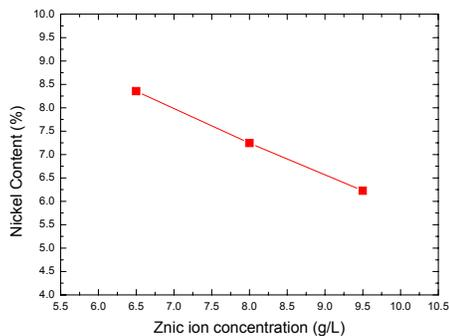
Fig. 3. The influence of the zinc ion concentration in the electrolyte on the nickel content of the coating.
