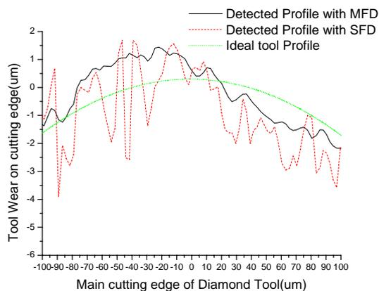
Fig.5. Results of the SFD and MFD detection method.
