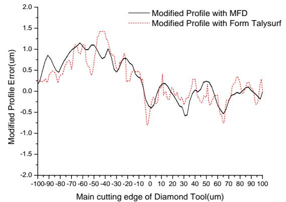
Fig.6. Comparison between the MFD-generated profile and profile measured by Form Talysurf.
