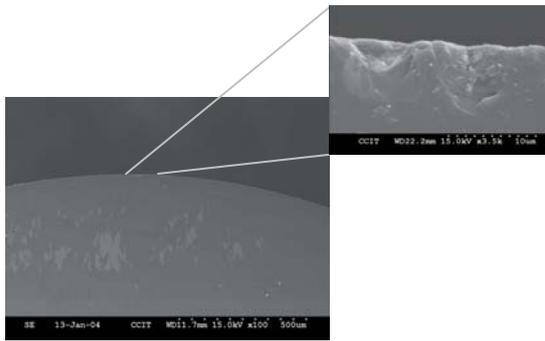
Fig.3. SEM image of round nose diamond tool.
