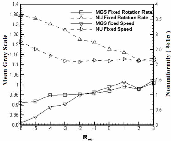
Fig.8. The effect of changing the distance from the wafer and polishing pad center while keeping rotational speed and its relative speed fixed,  $Q=150\text{ml/min}$  and  $\Omega = \omega = 30\text{rpm}$ .
