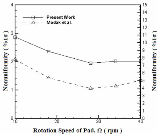
Fig.4. Variations of non-uniformity with pad rotation speed for wafer rotating speed of  $\omega=32$ rpm, slurry inject rate  $Q=150$  ml/min, injection position  $R_i/R_o=0\%$ , Non-uniformity data of Modak are also shown for comparison.
