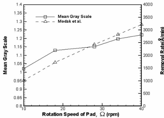
Fig.3. Variations of mean gray scale image with pad rotation speed for wafer rotating speed  $\omega=32$ rpm, flow rate  $Q=150$  ml/min, injection position  $R_i/R_o=0\%$ , Removal rate data of Modak are also shown for comparison.
