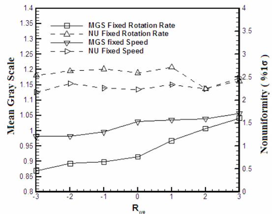
Fig.7. The effect of changing the distance from the wafer and polishing pad center while keeping rotational speed and its relative speed fixed,
