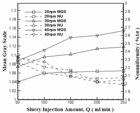
Fig.6. The optimal slurry injection amount experiment for the experiments conducted at  $\Omega = \omega = 20, 30$ , and  $40\text{rpm}$ ,  $IP = 0\%$
