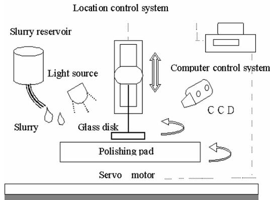
Fig.1. CMP experimental apparatus.
