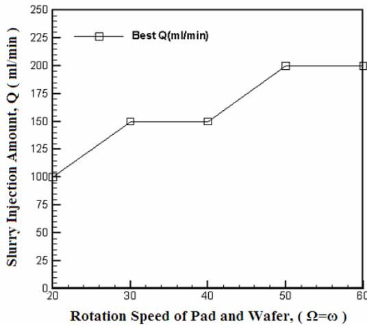
Fig.9. The best slurry amount for the wafer edge exceeds the polishing pad center for the slurry amount is set as  $R_i=R_{we}$ , the wafer edge exceeds the polishing pad center distance is set to be  $R_{we}=3\text{cm}$  while the
