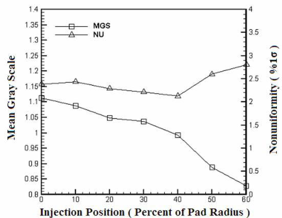
Fig.5. Mean gray scale (MGS) image and non-uniformity (NU) changes with varying injection position for  $Q=150$ ml/min, fixed the wafer rotating speed is  $\omega$  and the polishing pad rotating speed is  $\Omega$ , this
