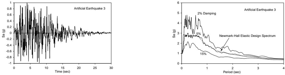
Fig.9 Artificial earthquakes generated from newmark-hall elastic design spectrum
