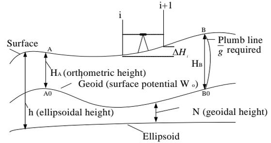
Fig.1. The scheme of precise leveling set-up between benchmark A and B
