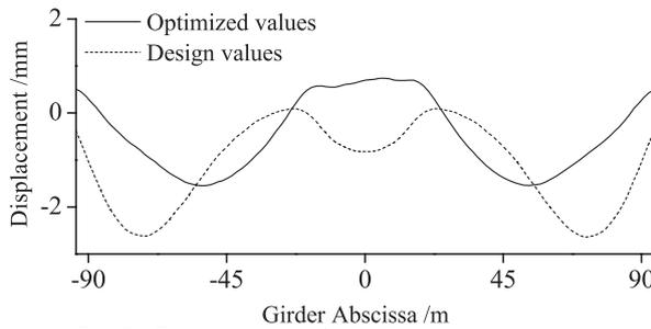
Fig.8. Comparison of girder displacements.
