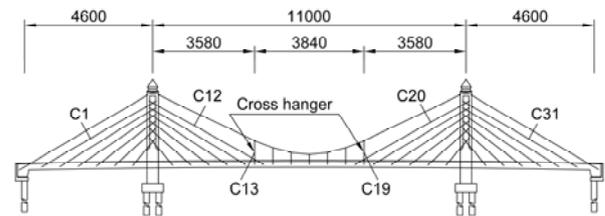
Fig. 5. Structural dimensions of the Zhuanghe Jianshe Bridge. (Units: cm)
