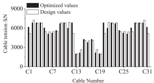
Fig.6. Comparison of cable tensions.
