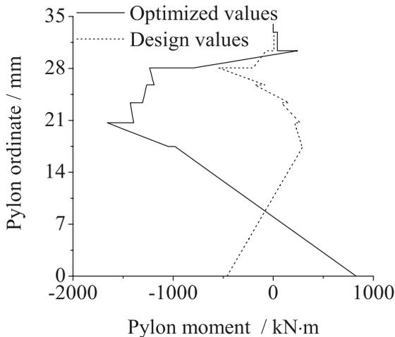
Fig.9. Comparison of pylon moments.
