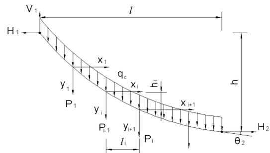
Fig. 3. Mechanical diagrammatic sketch of the main cable.
