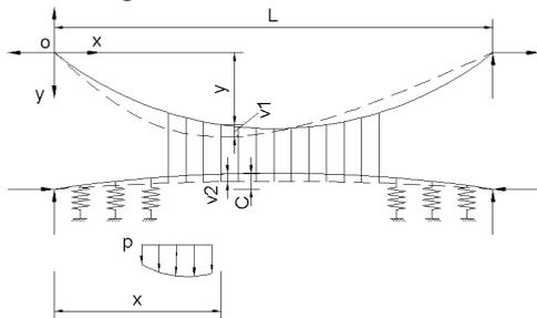
Fig. 2 Deflection theory of self-anchored cable-stayed-suspension bridges.
