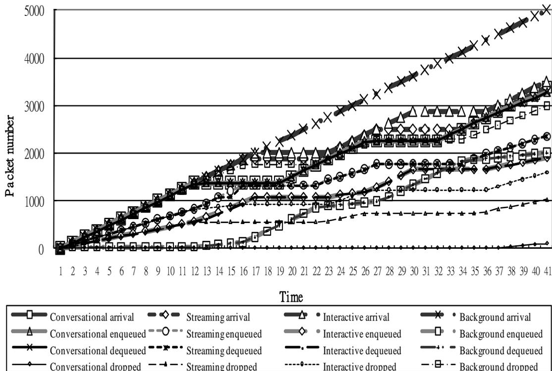
Fig. 7. Simulation results of UMTS traffic transmission in an intermittent pattern.
