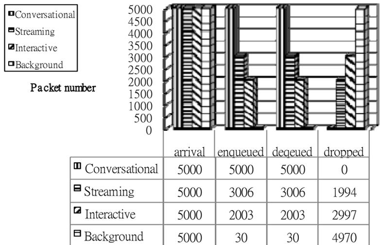
Fig. 6. Simulation results of all UMTS traffic in a continuous transmission pattern.
