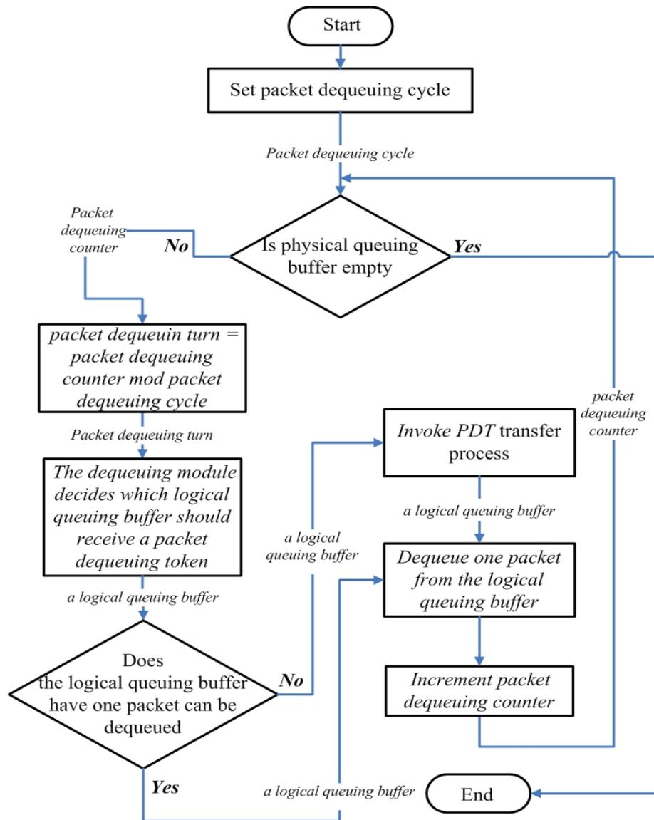
Fig. 4. The flowchart of the proposed weighted round robin packet dequeuing module.
