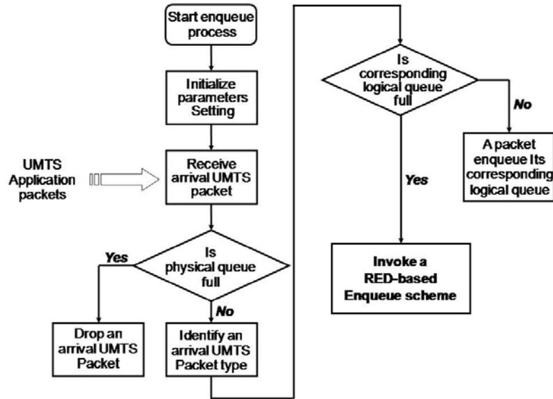
Fig. 3. The flowchart of the two-stage enqueueing process.
