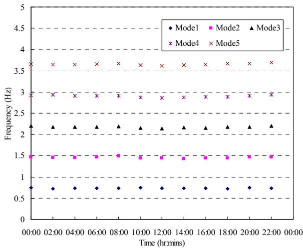
Fig.5. Variation of frequencies identified with time of day in torsional direction
