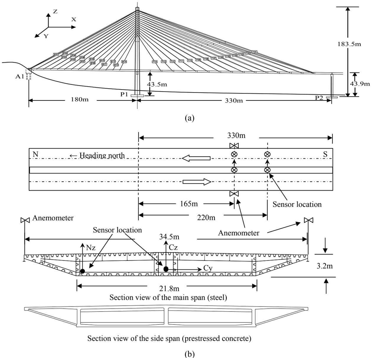
Fig.1. Layout of the Kao Ping Hsi cable-stayed bridge: (a) plane view; (b) sensor locations of the structural monitoring system.
