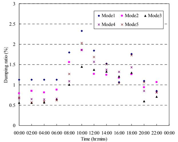
Fig.6. Variation of damping ratios identified with time of day in torsional direction
