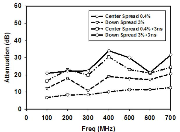
Fig.4. Attenuation values of the  $\delta = 3\%$  down-spread and the  $\delta = \pm 0.4\%$  center-spread schemes, both with and without an additional rise/fall time of 3 ns;  $f_c = 100$  MHz.
