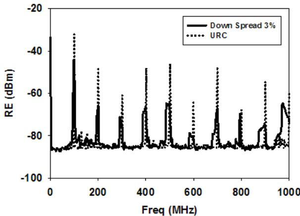
Fig.2. Radiated emissions from the antenna excited by the down-spread SSC with  $\delta = 3\%$  and the corresponding URC (or SSC with  $\delta = 0$ );  $f_c = 100$  MHz.
