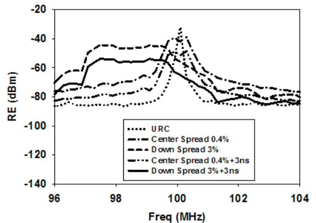
Fig.3. RE of spread SSCs with two different spreading schemes and with or without a 3 ns longer rise/fall time at fundamental frequency 100 MHz.
