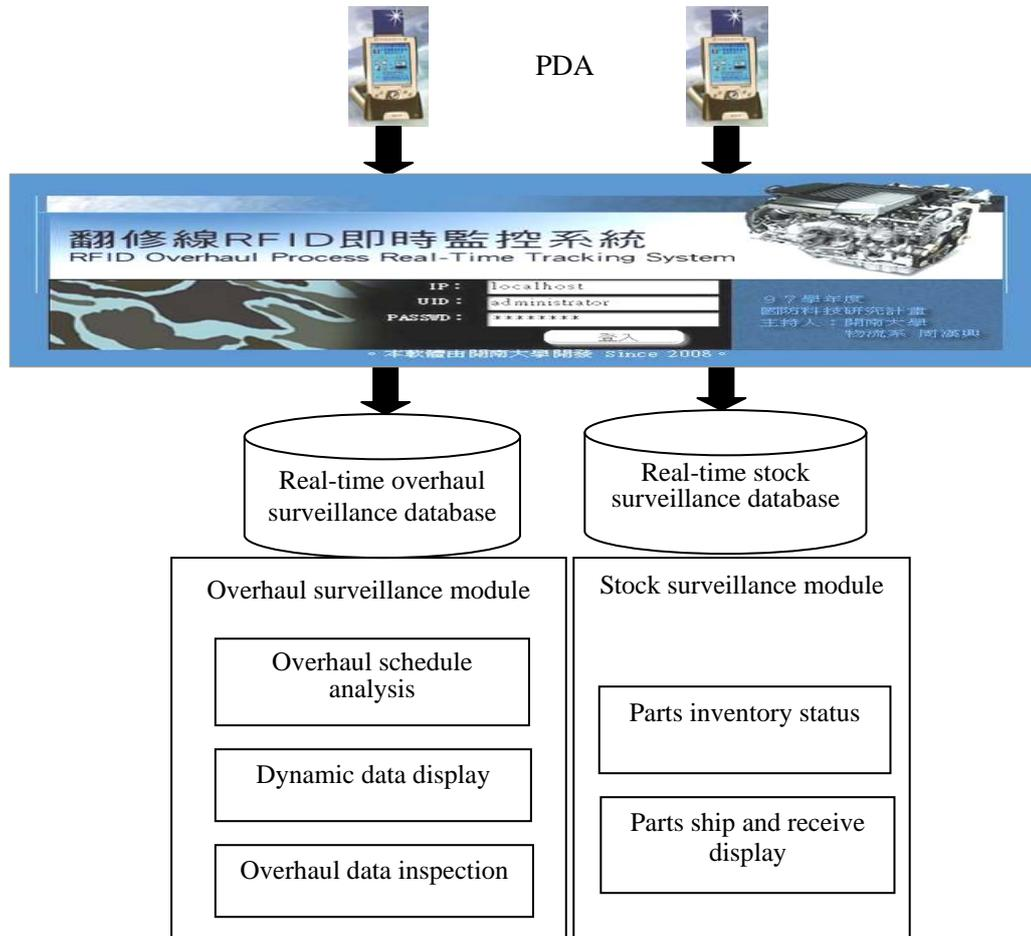
Figure 5. Real-time surveillance system framework
