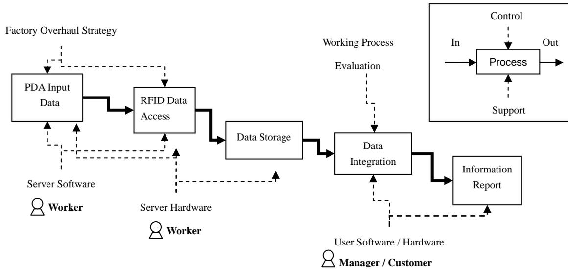
Figure 3. The Input-Process-Output relationship between the PDA, RFID, Server and the User.
