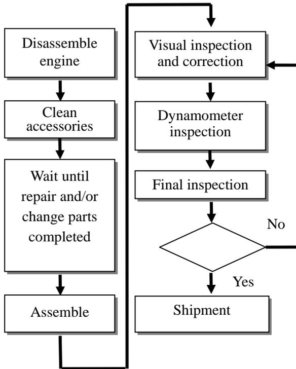
Figure 1. Engine overhaul procedures.
