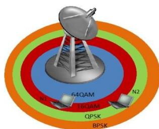
Fig. 5. Four modulations in WiMAX/LTE.
