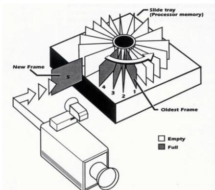
Fig. 6. Slide tray (processor memory).
