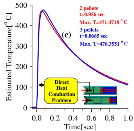
Fig. 9. (a) Experimentally measured temperature-time curves at  $x=L$  for properly ignited two pellets and three pellets of delay columns. (b) Estimated time-varying heat flux-time curves at  $x=0$  by means of input estimation method with the measured temperatures in (a) as input. (c) Estimated temperature-time curves at  $x=L$  by means of direct heat conduction problem with the time-varying heat flux in (b) as input.
