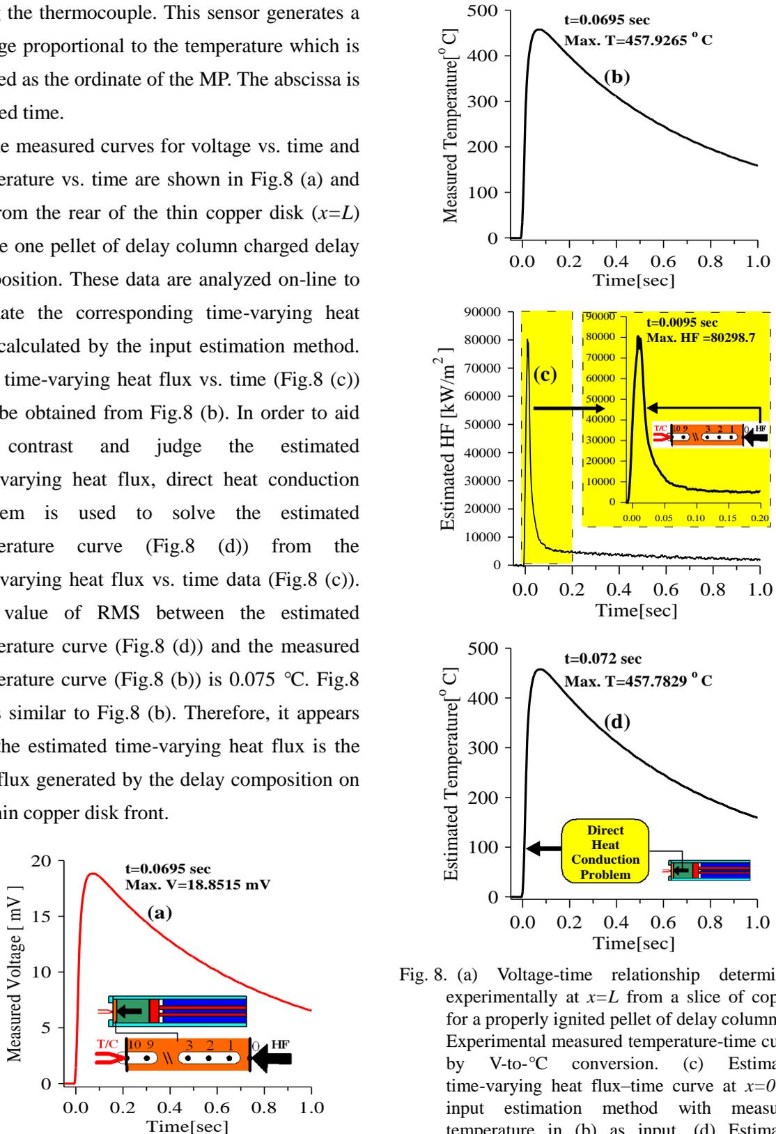
Fig. 8. (a) Voltage-time relationship determined experimentally at  $x=L$  from a slice of copper for a properly ignited pellet of delay column. (b) Experimental measured temperature-time curve by V-to- $^{\circ}\text{C}$  conversion. (c) Estimated time-varying heat flux-time curve at  $x=0$  by input estimation method with measured temperature in (b) as input. (d) Estimated temperature-time curve at  $x=L$  by direct heat conduction problem with estimated time-varying heat flux in (c) as input.
