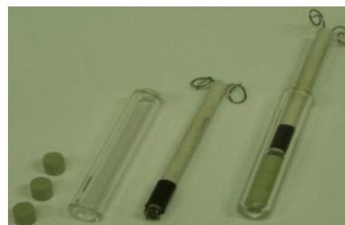
Fig. 7. Three delay columns loaded in the crystal tube.
