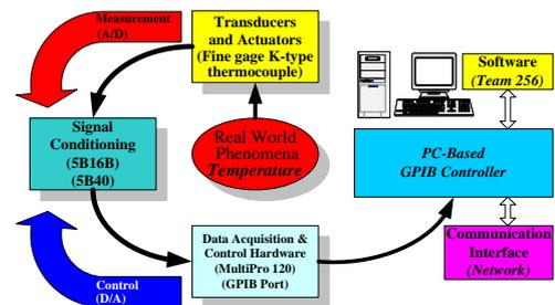
Fig. 3. Schematic diagram of the experimental facility.
