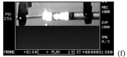
Fig. 10. The snap shots of combustion propagation by means of Kodak Ektapro hi-spec motion analyzer for three pellets of delay columns loaded in the crystal tube. (a) The first pellet of delay column is ignited. (b) The second pellet of delay column is ignited. (c) The third pellet of delay column is ignited. (d) The third pellet of delay column burns at the extreme end. (e) The output of combustion flame is violent. (f) The output of combustion flame weakens.
