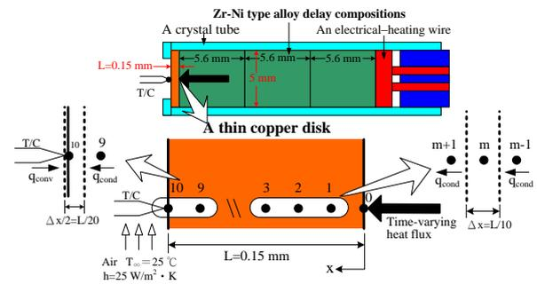
Fig. 1. Physical model of one dimensional inverse heat conduction problem (geometry and coordinates).
