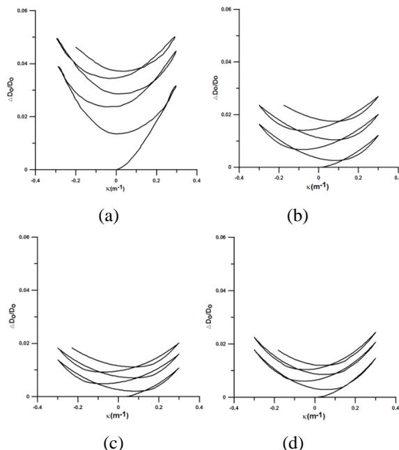
Fig. 16. Cyclic ovalization ( $\Delta D_o/D_o$ ) - curvature ( $\kappa$ ) for Tube B. (a) Experiment result, (b) theoretical analysis by the endochronic theory combined with the principle of virtual work, (c) theoretical analysis by ANSYS and (d) theoretical analysis by ABAQUS
