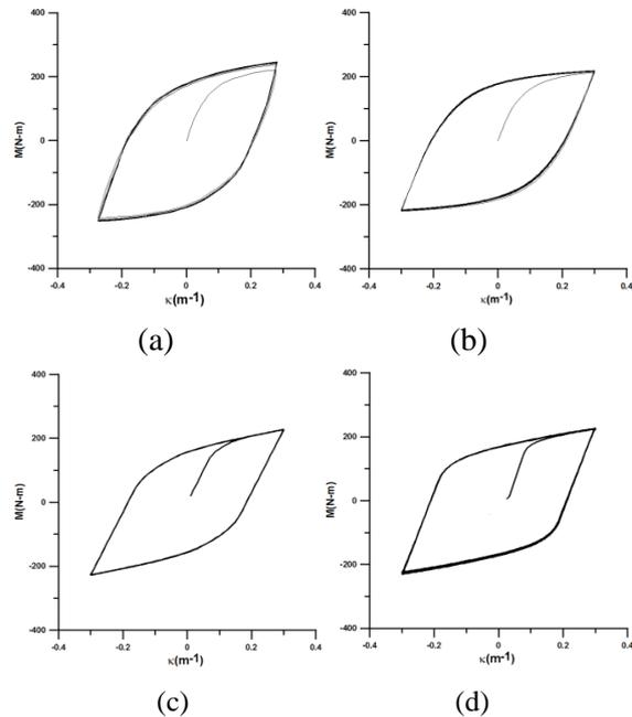
Fig. 13. Cyclic moment ( $M$ ) - curvature ( $\kappa$ ) for Tube A. (a) Experiment result, (b) theoretical analysis by the endochronic theory combined with the principle of virtual work, (c) theoretical analysis by ANSYS and (d) theoretical analysis by ABAQUS
