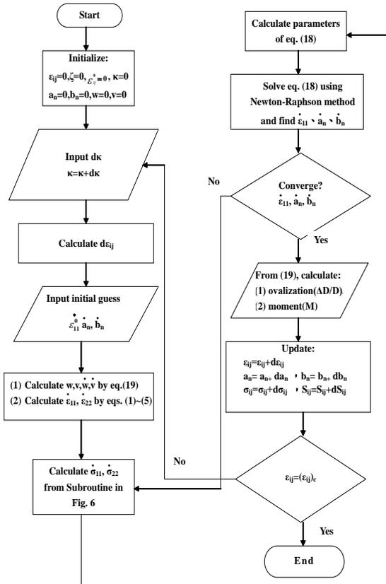
Fig. 6. Flow chart of the numerical solution procedure
