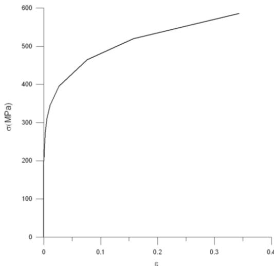
Fig. 8. Multilinear segments of the stress-strain relationship for 316L stainless steel
