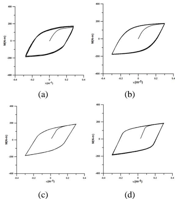
Fig. 14. Cyclic moment ( $M$ ) - curvature ( $\kappa$ ) for Tube B. (a) Experiment result, (b) theoretical analysis by the endochronic theory combined with the principle of virtual work, (c) theoretical analysis by ANSYS and (d) theoretical analysis by ABAQUS
