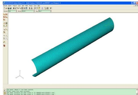
Fig. 11. Mesh of the finite element ABAQUS
