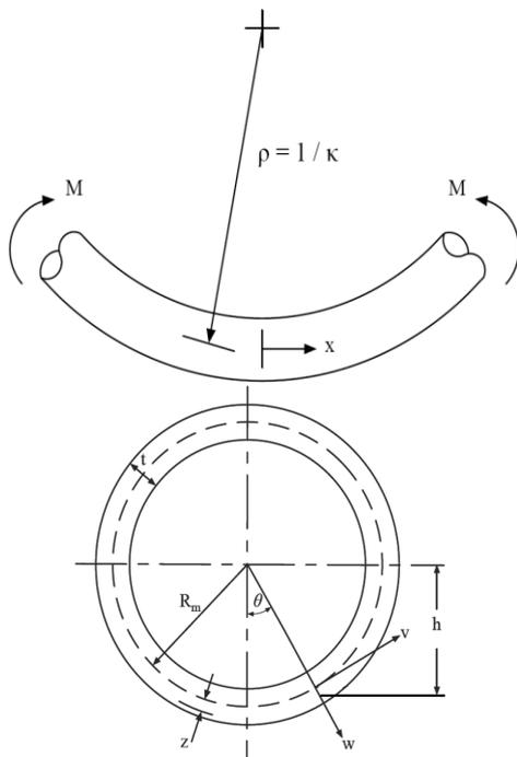
Fig. 5. Problem geometry of circular tube subjected to pure bending
