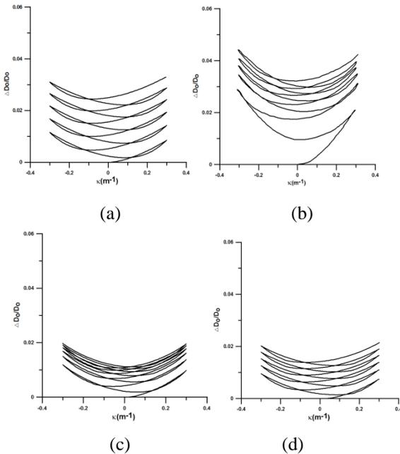
Fig. 15. Cyclic ovalization ( $\Delta D_o/D_o$ ) - curvature ( $\kappa$ ) for Tube A. (a) Experiment result, (b) theoretical analysis by the endochronic theory combined with the principle of virtual work, (c) theoretical analysis by ANSYS and (d) theoretical analysis by ABAQUS
