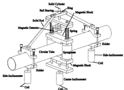
Fig. 3. Schematic drawing of the COMA
