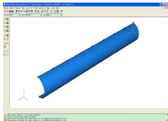
Fig. 12. Boundary condition of the finite element ABAQUS
