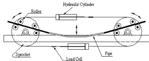
Fig. 2. Schematic drawing of the tube-bending device
