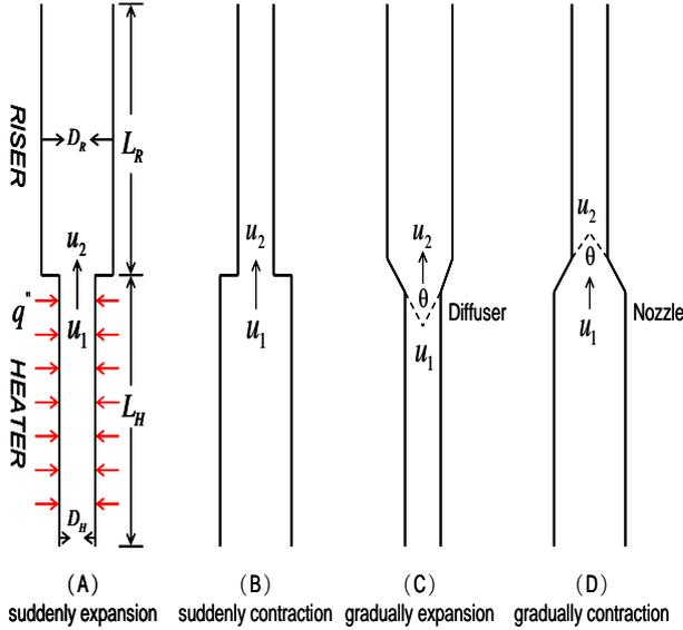
Fig. 1. The fundamental formation types of the heater-riser system.
