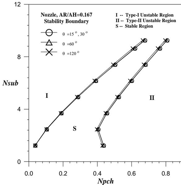
Fig. 8. The effects of the included angle on the stability of a nozzle system at an area ratio  $A_R / A_H = 0.167$ .
