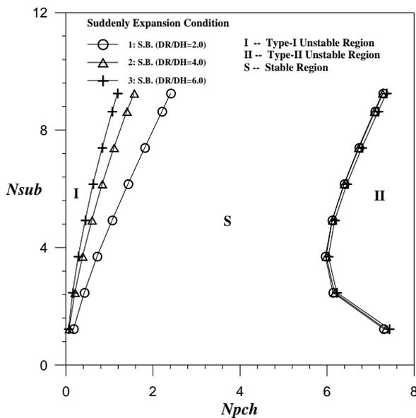
Fig. 3. The effect of the suddenly expansion structure on the stability of the two-phase natural circulation system.
