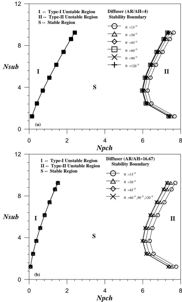
Fig. 6. The effects of the included angle on the stability of a diffuser system under different area ratios: (a)  $A_R/A_H = 4$ , (b)  $A_R/A_H = 16.67$
