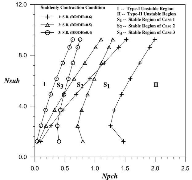
Fig. 4. The effect of the suddenly contraction structure on the stability of the two-phase natural circulation system.
