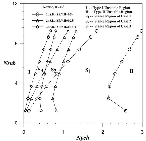
Fig. 9. The effect of the area ratio on the stability of a nozzle system at an included angle  $\theta=15^\circ$ .
