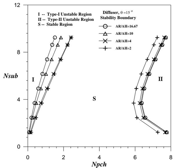
Fig. 7. The effects of the area ratio on the stability of a diffuser system at an included angle  $\theta = 15^\circ$ .
