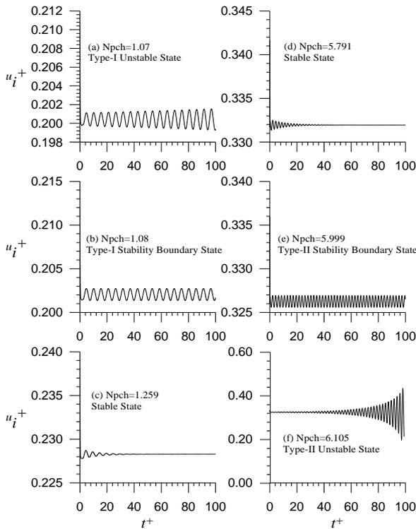
Fig. 2. Transient responses following a perturbation in the inlet velocity of the heater by changing the heating power at  $N_{sub} = 4.936$  for a natural circulation ABWR.
