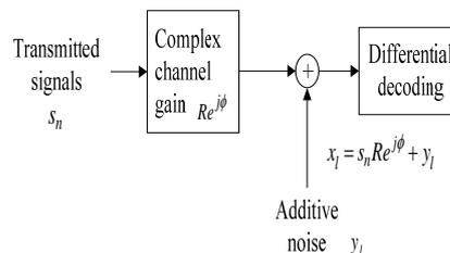
Fig.1. Model of fading channel communications.
