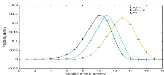
Fig. 8. The pdf of the diversity combiner output energy with MESC.
