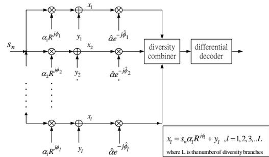
Fig. 3. The block diagram of a diversity combiner.
