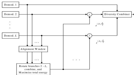
Fig.4. The block diagram of a misalignment-free diversity combiner.
