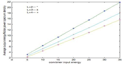
Fig. 5. the output energy vs. total input energy of the diversity combiner without MESC.
