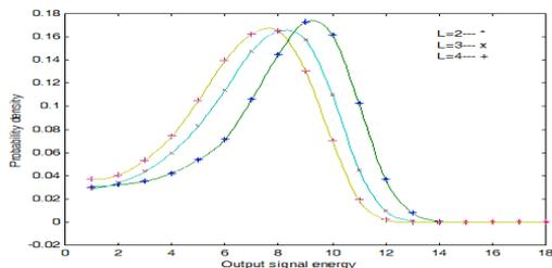
Fig. 7. The pdf of the diversity combiner output energy without MESC.
