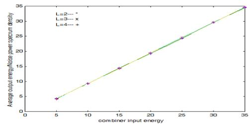
Fig. 6. The output energy vs. total input energy of the diversity combiner with MESC.
