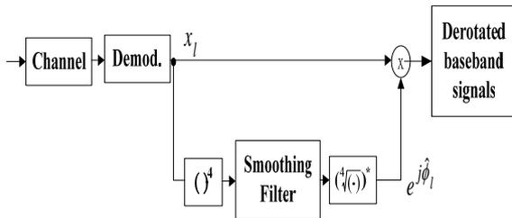
Fig. 2. The nonlinear phase estimator for QPSK modulated signals.
