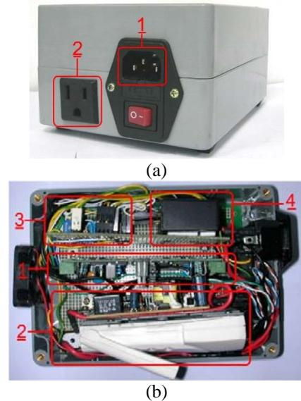
Fig. 8. (a) Outer appearance of WMM, (b) Inner connection of the units in WMM.
