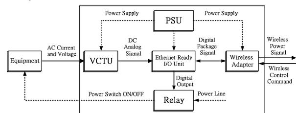
Fig. 7. Functional blocks of the Wireless Monitoring Module (WMM) [29].
