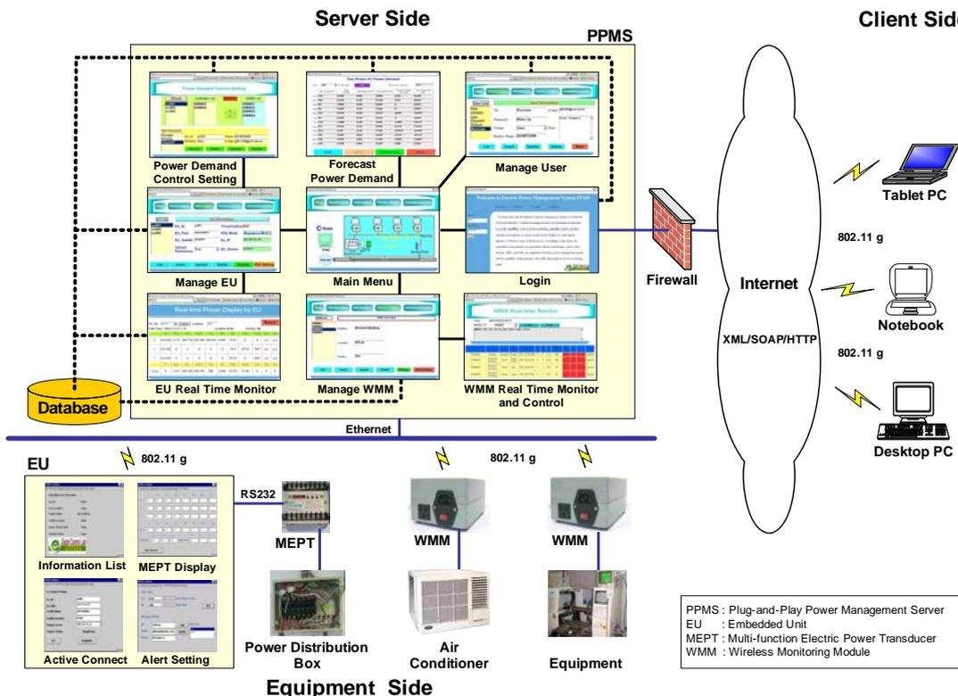
Fig. 9. Snapshot of the integration test of the prototype DSPMS.
