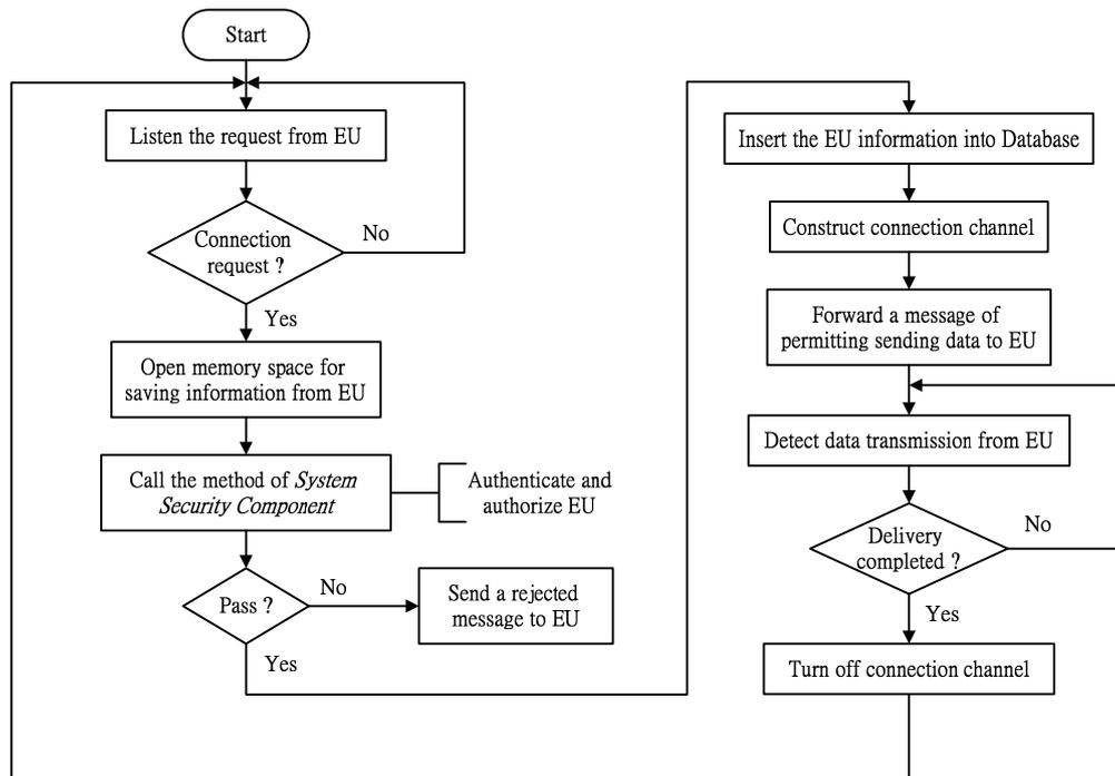
Fig. 2. The operation flow of the Plug-and-Play component.
