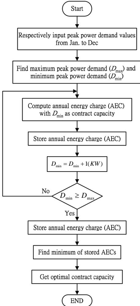
Fig. 3. The operational flow of the optimal contract capacity prediction mechanism.
