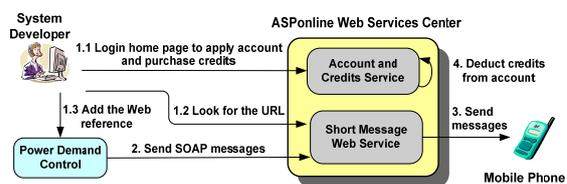
Fig. 4. Mobile phone text message delivery mechanism based on Web service technology.
