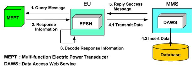
Fig. 5. Message transmission between an embedded unit and the MMS.
