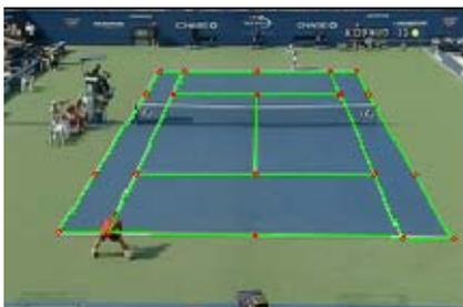
Fig. 6. Court line detection result (highlighted in green).
