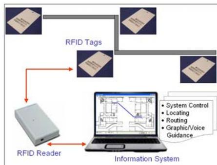
Fig.1. System architecture of using passive RFID for indoor guidance.
