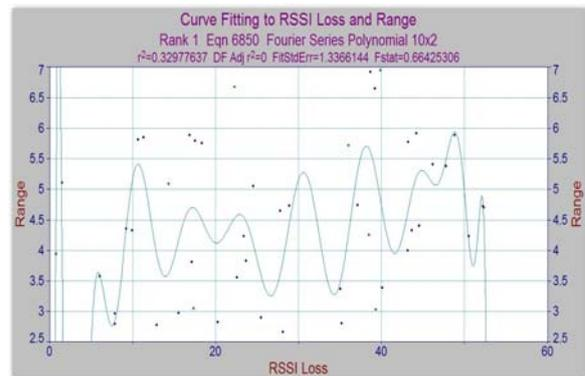
Fig.14. Best-fitting curve model for range estimation.
