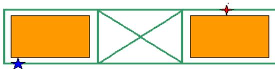
Fig.2. Scenario of “available” paths between two nodes (The symbols of cross, star and circle represent the start, end and way points, respectively).
