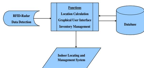
Fig.16. System architecture for RFID-Radar locating and management.
