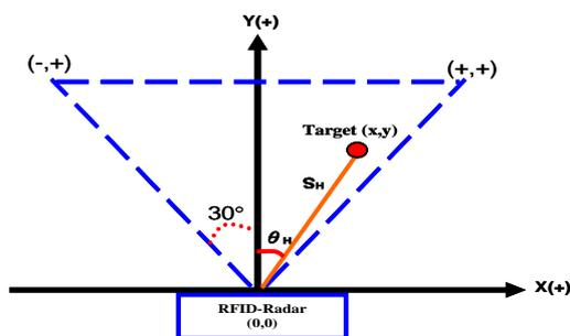
Fig.19. Self-defined 2D local coordinate system for RFID-Radar operation.
