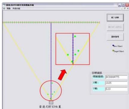
Fig.23. GUI displays the item checking result (with the locations magnified).
