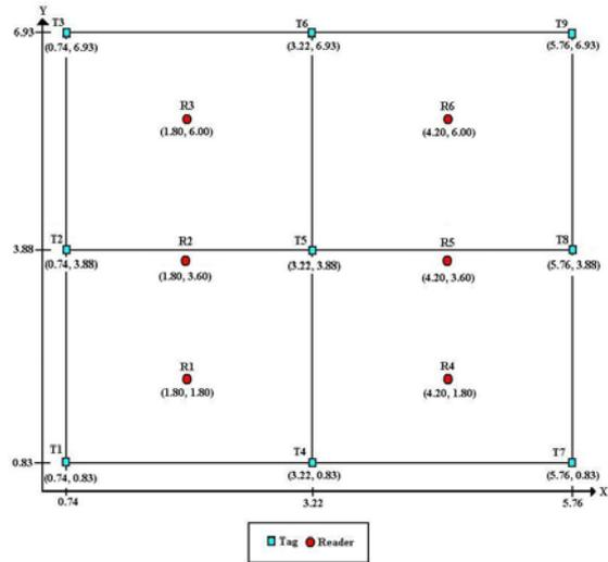
Fig.12. Test field design for active RFID.
