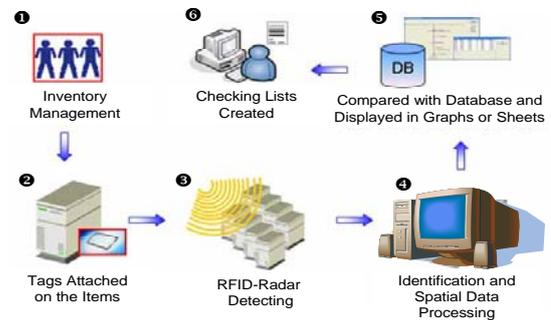
Fig.15. Inventory management procedure with the RFID-Radar system
