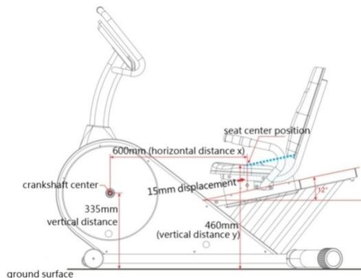
Fig.2 Position adjustment schematic for the experiment.
