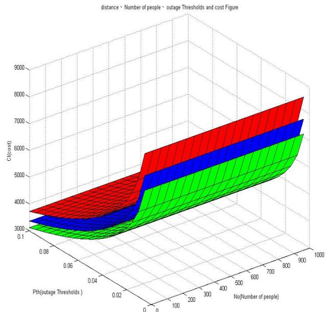
Fig. 2. The curves among cost utility, mobile user numbers, and threshold outage probability.
