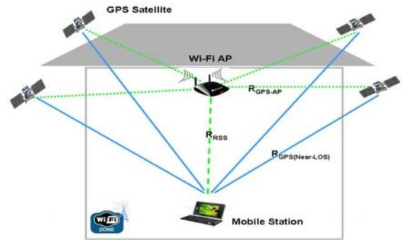
Fig. 4. The Range Composition of WiFi/GPS Hybrid Positioning.
