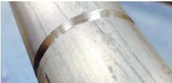
Fig. 1. Picture of a tube with a circumferential sharp notch.
