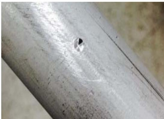
Fig. 2. Picture of a tube with a local sharp notch.
