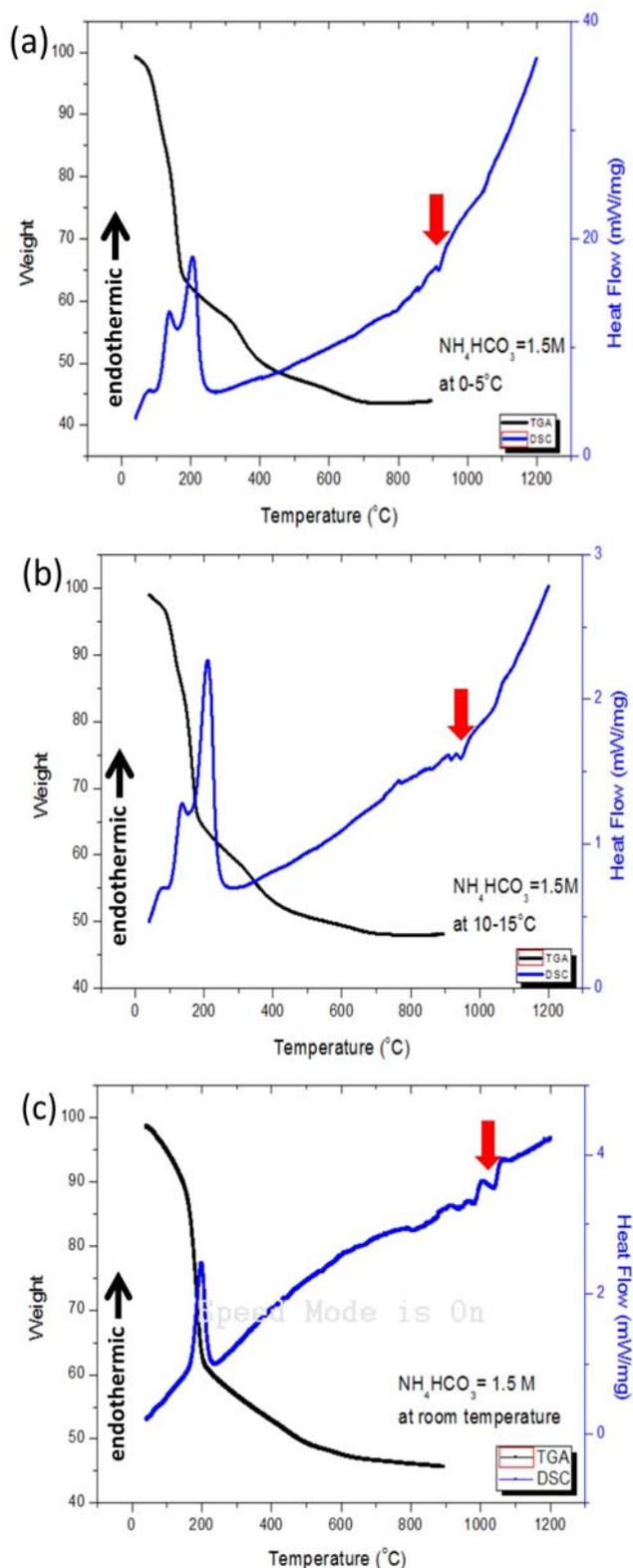
Fig. 1. DSC-TG curves of the Nd:YAG precursor samples precipitated at various temperature: (a) 0-5 $^{\circ}$ C; (b) 10-15 $^{\circ}$ C and (c) 25 $^{\circ}$ C.
