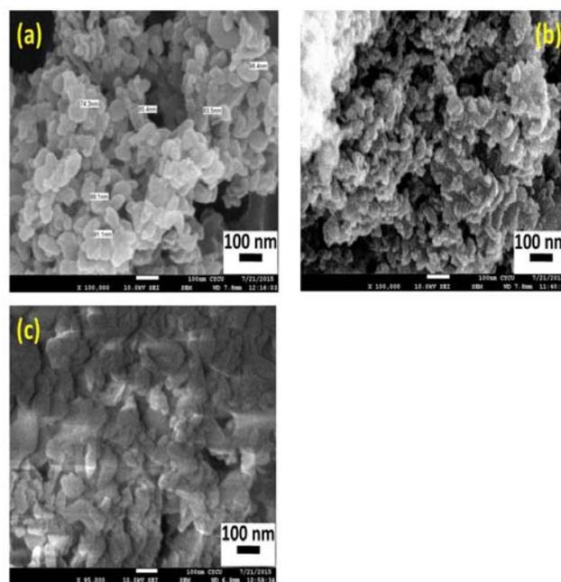
Fig. 6. SEM micrographs of the Nd:YAG precursor co-precipitated at 20 °C and various precipitating agent concentration: (a) 1 M; (b) 1.5 M and (c) 2 M.
