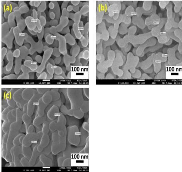
Fig. 7. SEM micrographs of the Nd:YAG precursor co-precipitated at 10 °C , various precipitating agent concentration and calcined at 1200°C: (a) 1 M; (b) 1.5 M and (c) 2 M.
