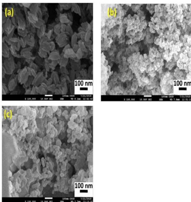
Fig. 5. SEM micrographs of the Nd:YAG precursor co-precipitated at 10 °C and various precipitating agent concentration: (a) 1 M; (b) 1.5 M and (c) 2 M.
