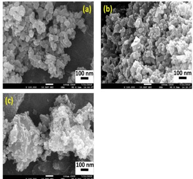
Fig. 4. SEM micrographs of the Nd:YAG precursor co-precipitated at 0 °C and various precipitating agent concentration: (a) 1 M; (b) 1.5 M and (c) 2 M.
