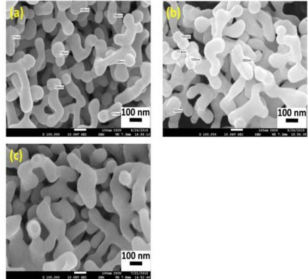
Fig. 8. SEM micrographs of the Nd:YAG precursor co-precipitated at 20 °C , various precipitating agent concentration and calcined at 1200°C: (a) 1 M; (b) 1.5 M and (c) 2 M.
