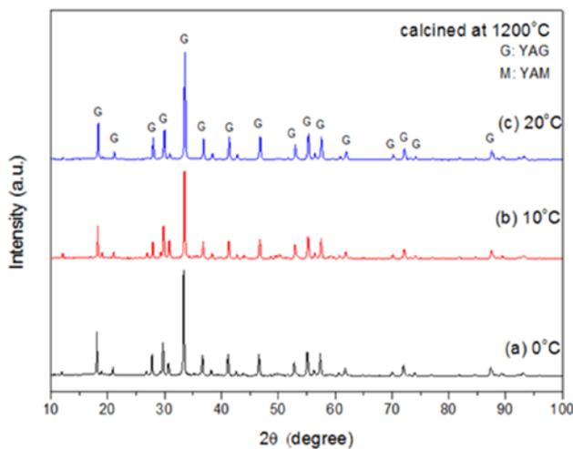
Fig. 3. XRD spectra of Nd:YAG precursor precipitated at various temperature and calcined at 1200°C when the precipitating agent concentration was 2 M: (a) 0°C; (b) 10 °C and (c) 20°C.
