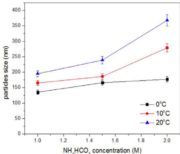
Fig. 9. Relationship between particles size of Nd:YAG precursors calcined at 1200 °C and precipitating agent concentration at different co-precipitated temperature.
