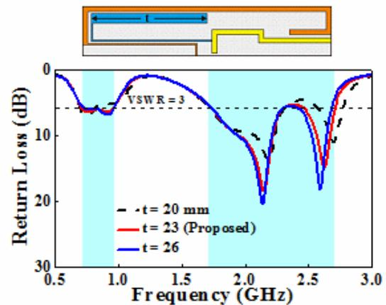
Fig. 5. Simulated return loss as a function of the length  $t$  of the coupling section of the rotated U-shaped strip.
