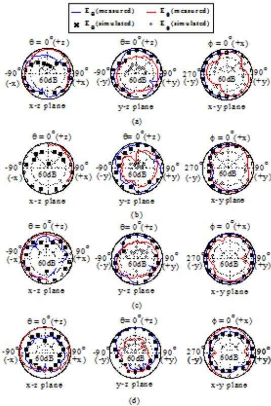
Fig. 8. Measured and simulated radiation patterns of the proposed antenna: (a)  $f = 740$  MHz, (b)  $f = 900$  MHz, (c)  $f = 2100$  MHz, and (d)  $f = 2610$  MHz.
