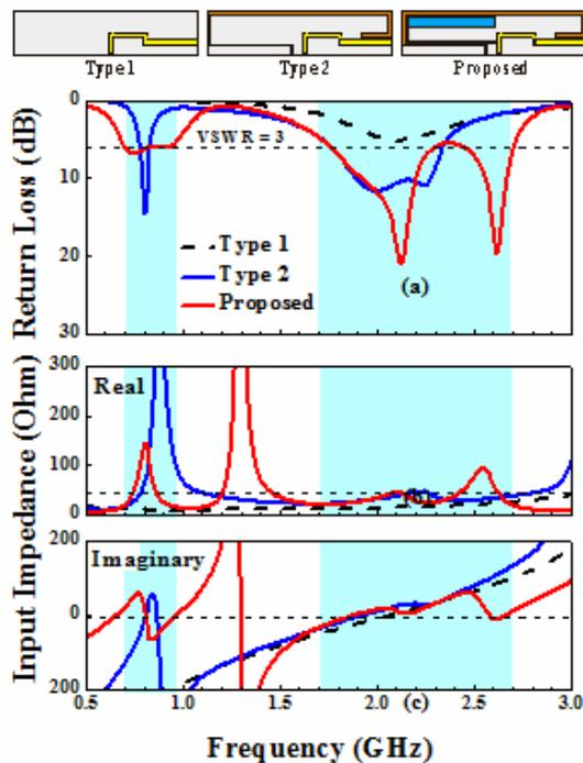
Fig. 4. Simulated S parameters for the proposed WLAN MIMO antenna array, the Type1 design, and the Type2 design.
