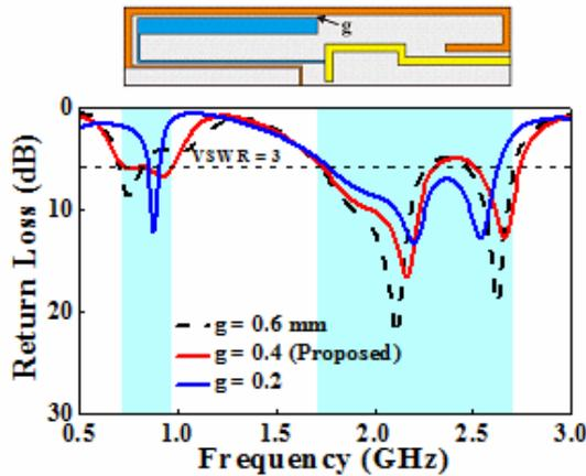
Fig. 6. Simulated return loss as a function of the width  $g$  of the coupling gap.
