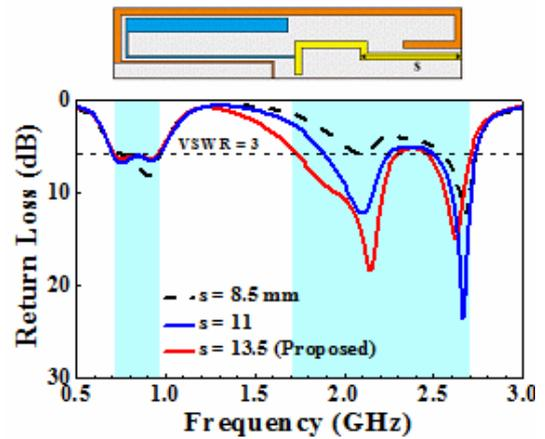
Fig. 7. Simulated return loss as a function of the length  $s$  of the feeding strip.
