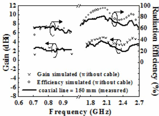
Fig. 9. Simulated and measured radiation efficiency and antenna gain of the proposed antenna.
