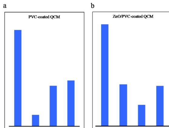
Fig.5. Response patterns of four compounds obtained from (a) PVC-coated and (b) ZnO/PVC-coated QCMs. Four compounds (from left to right) : *m*-xylene, octane, butyl acetate and butanol
