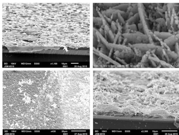
Fig.2. SEM images of (a) PVC film coated on QCM, (b) ZnO powders, and (c, d) ZnO/PVC film coated on QCM
