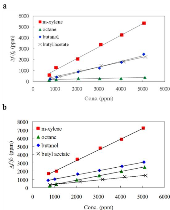
Fig.4. Calibration curves of four compounds tested with (a) PVC-coated and (b) ZnO/PVC-coated QCMs
