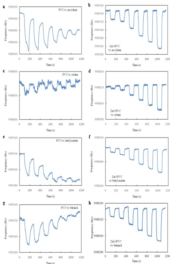
Fig.3. Response curves of PVC and ZnO/PVC coated QCM sensors at the various concentrations of (a, b) *m*-xylene, (c, d) octane, (e, f) butyl acetate, and (g, h) butanol
