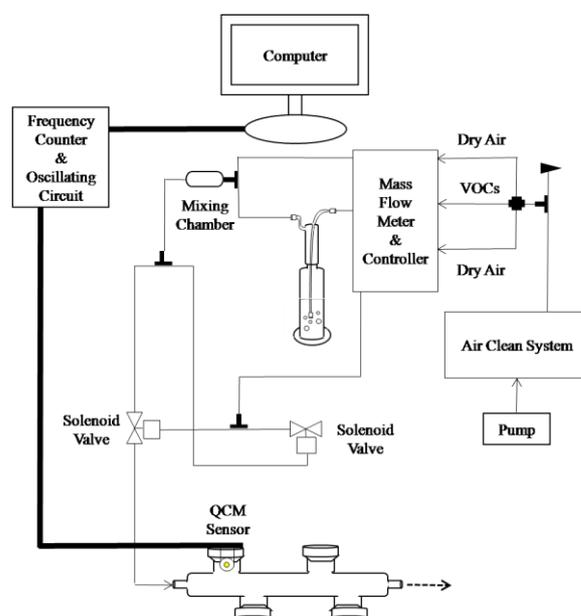
Fig.1. Schematic diagram of gas sensor measurement system
