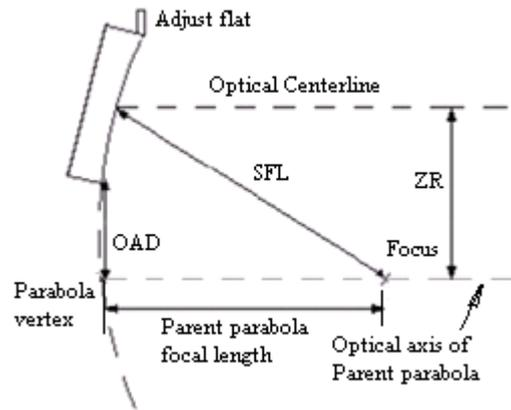
Fig.1 The off-axis parabolic mirror
