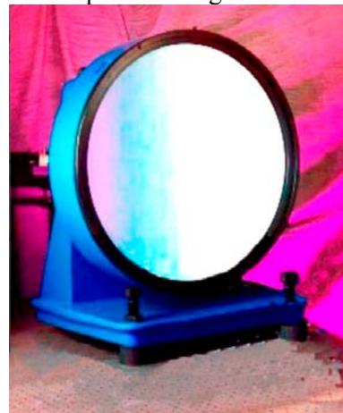
Fig.5 The OAP mirror under test
