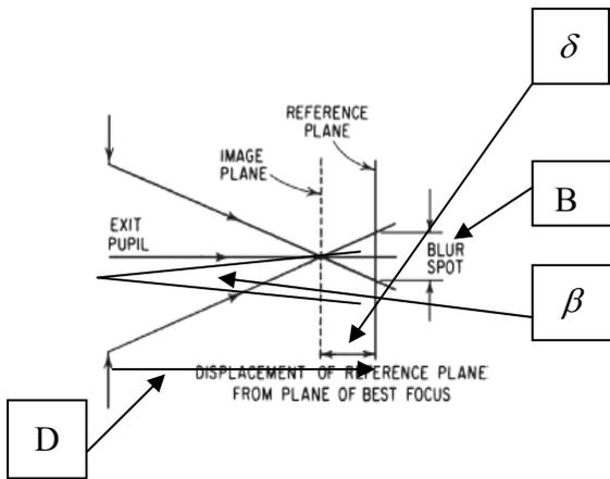
Fig.2 Depth of focus  $\delta$
