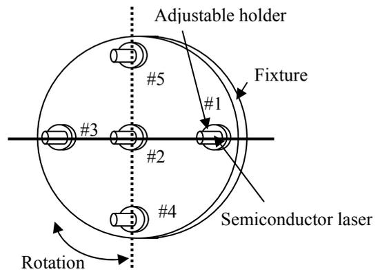
Fig.4 The rotational mechanism
