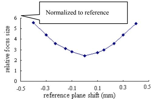
Fig.7 Focus size when reference plane shifted
