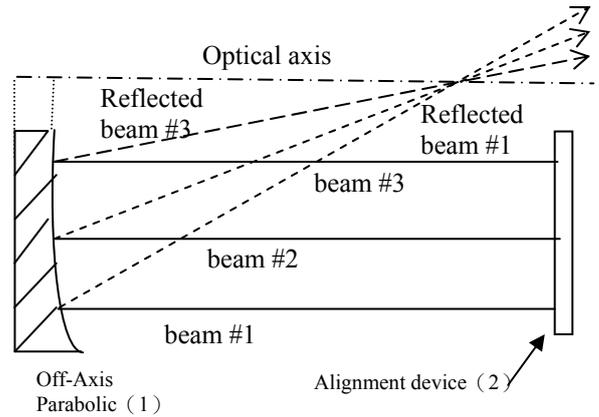
Fig.3 The optical alignment system
