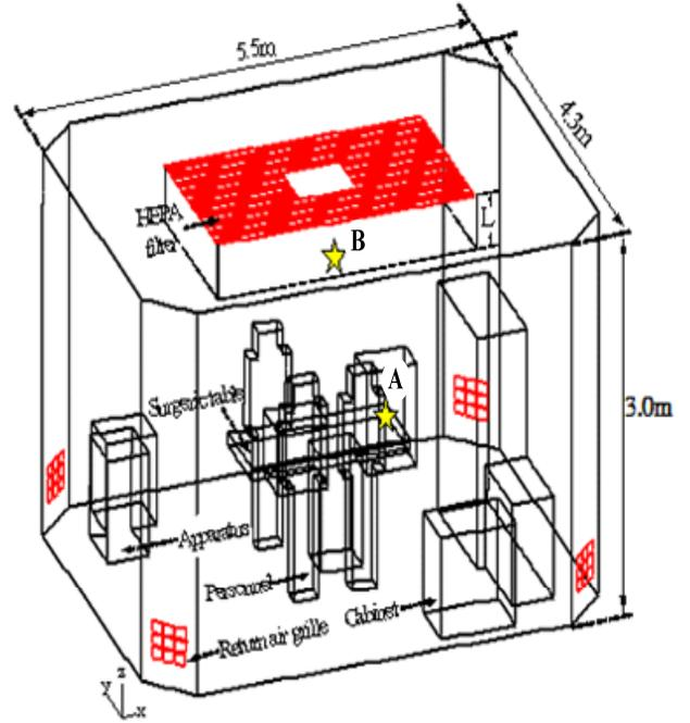
Fig. 2. Geometric model of the operation room.
