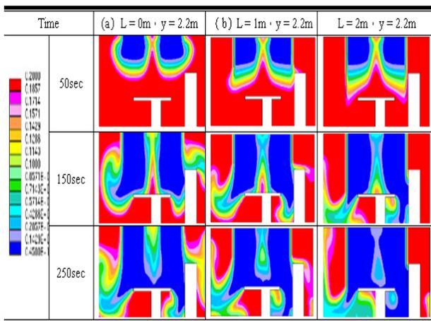
Fig. 4. Concentration field for different curtain length (at  $y = 2.2$  m).
