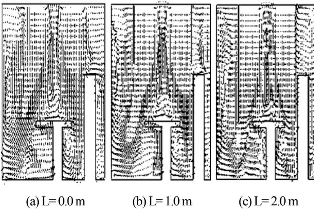
Fig. 3. Velocity vectors for different curtain length (at  $y = 2.2$  m).
