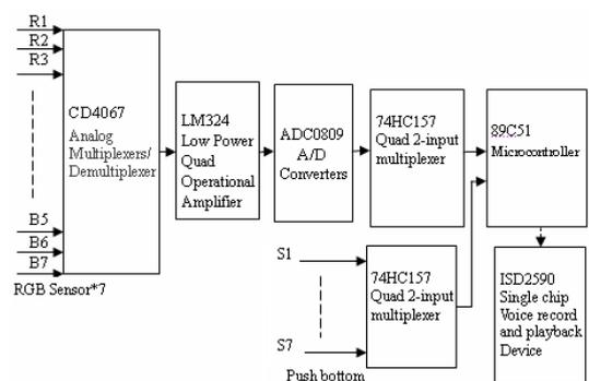
Fig.4. Seven color ball sensors measurement system.
