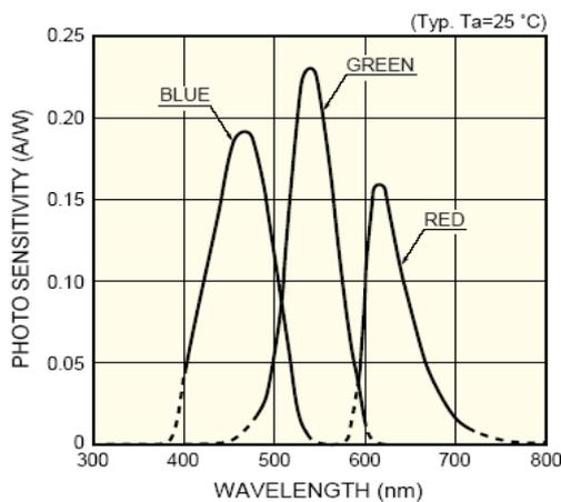
Fig.7. The spectral response of RGB Sensor.
