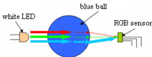
Fig.3. Ray trace of the tested color by color ball test device.
