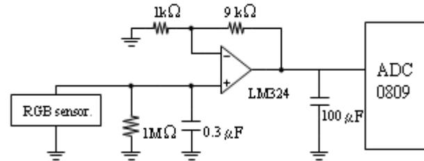
Fig.1. photodiode operation circuit.
