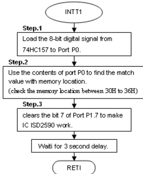
Fig.6. (b) Interrupts 1 subprogram flow chart.
