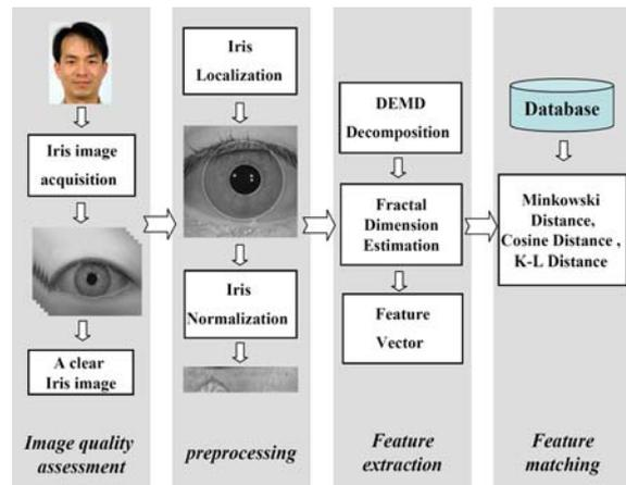
Fig. 1. Block diagram of the proposed iris recognition system.
