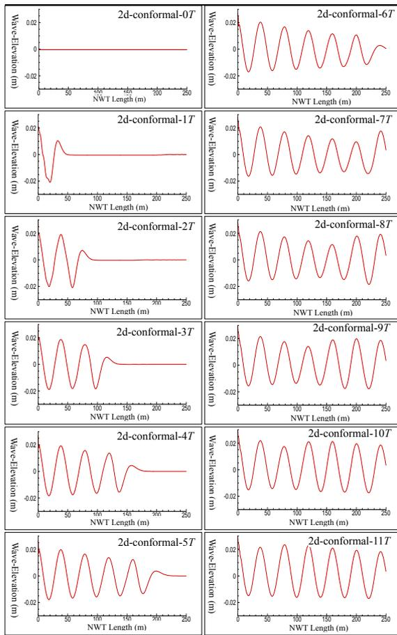
Fig. 5. Wave profile variation from 0 to 11T for conformal grid case
