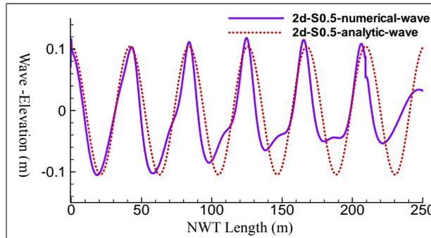
Fig.11. Comparisons of numerical and analytic wave-profiles for stroke value  $S_{0.5}$
