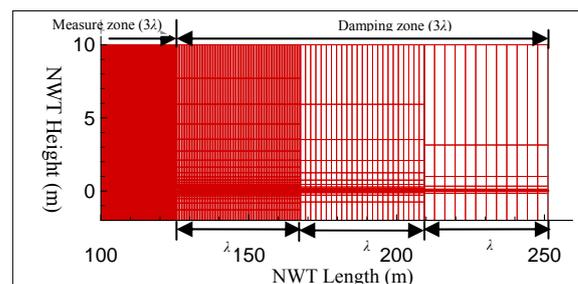
Fig. 6. Non-conformal grid allocation in 2D NWT
