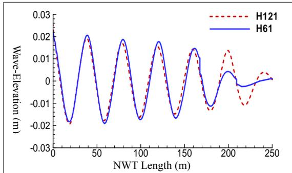
Fig. 3. The comparison of wave profiles with  $N_H=121$  and  $N_H=61$  at wave period =  $6T$ .
