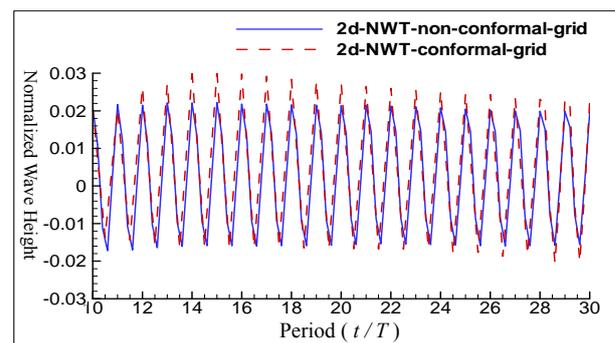
Fig. 9. Comparison of normalized wave profiles given with conformal and non-conformal grids in damping zone/measure position  $x=40m$
