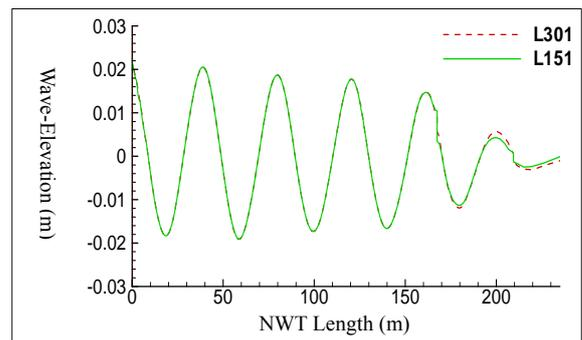
Fig. 2. The comparison of wave profiles with  $N_\lambda=301$  and  $N_\lambda=151$  at wave period =6T.
