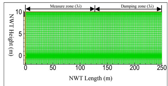
Fig. 4. Conformal grid allocation in 2D NWT
