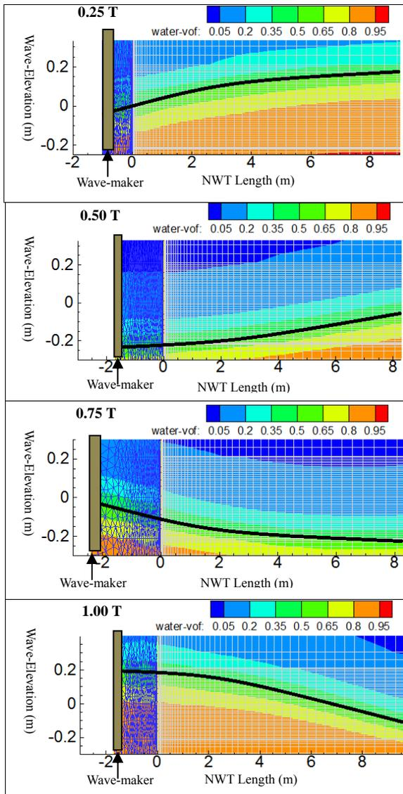
Fig. 1. The dynamic mesh motion of the piston-type wave-maker
