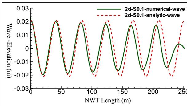
Fig. 13. Comparisons of numerical and analytic wave-profiles for stroke value  $S_{0.1}$
