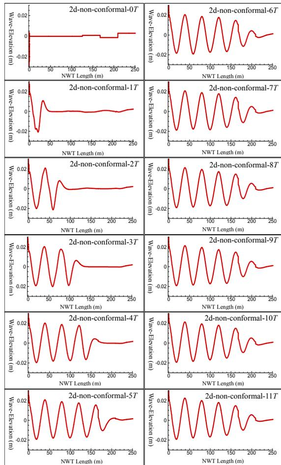
Fig. 7. Wave-profile variation from 0 to 11T for non-conformal grid case
