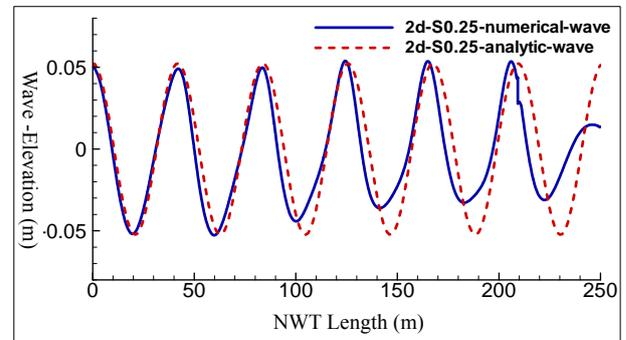
Fig. 12. Comparisons of numerical and analytic wave-profiles for stroke value  $S_{0.25}$
