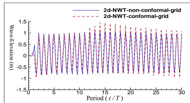
Fig. 8. Comparison of wave profiles given with conformal and non-conformal grids in damping zone/measure position  $x=40m$
