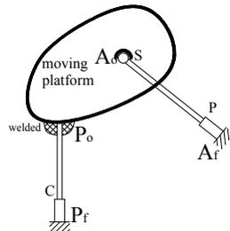
Fig. 3. Cylindrical joint and single landmark.
