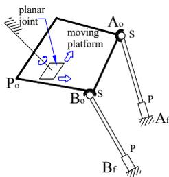
Fig. 4. Planar joint and two landmarks.
