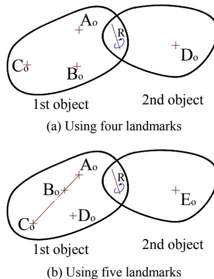
Fig. 12. Two objects connected by revolute joint.
