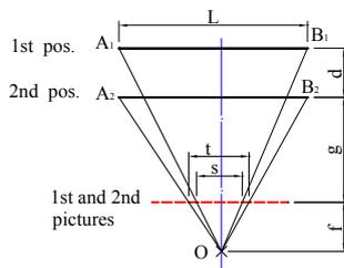
Fig. 11. Illustration of camera calibration.
