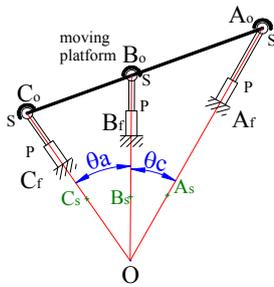
Fig. 9. Analogous mechanism with three collinear landmarks.
