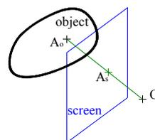
Fig. 1. Camera system with single landmark.
