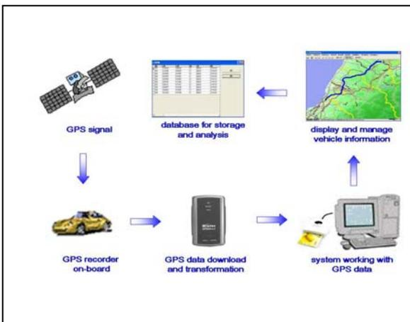
Fig. 9. Operation flow for vehicular management system
