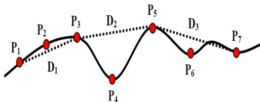
Fig. 2. Chord length computation using fixed data interval (where the data interval is set to be 2)
