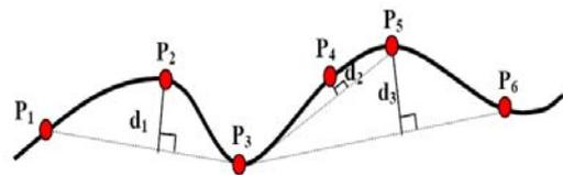
Fig. 3. Chord length computation based on vertical offset
