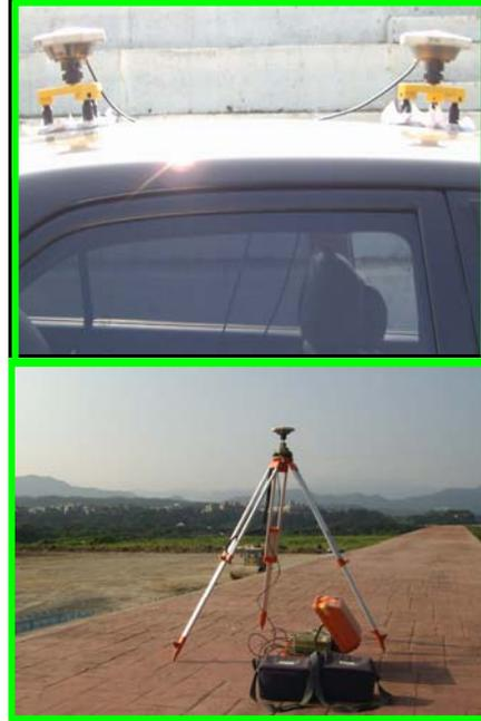
Fig. 6. GPS receivers set up for data collection and accuracy test
